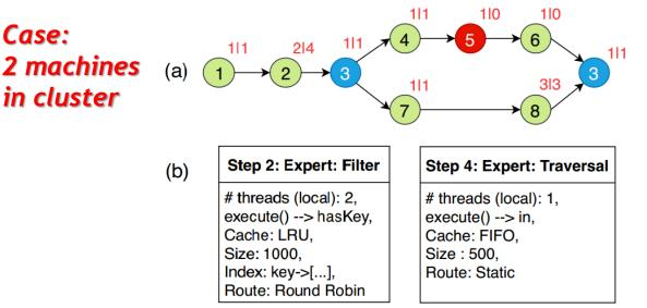
Figure 7. (a) adaptive parallelism at step-level; (b) an expert example.
