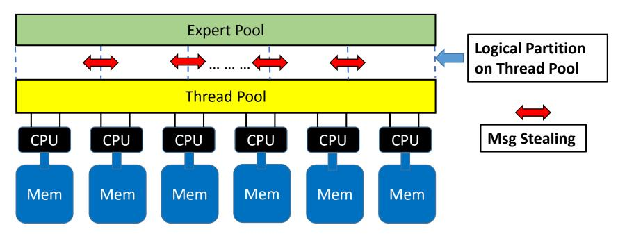
Figure 8. Core bind and load balancing in Grasper.
