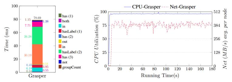
Figure 10. (a) The query latency breakdown of IC4 on LDBC by Grasper; (b) CPU and network utilization of Grasper for the mixed workload {IS1-IS4}.
