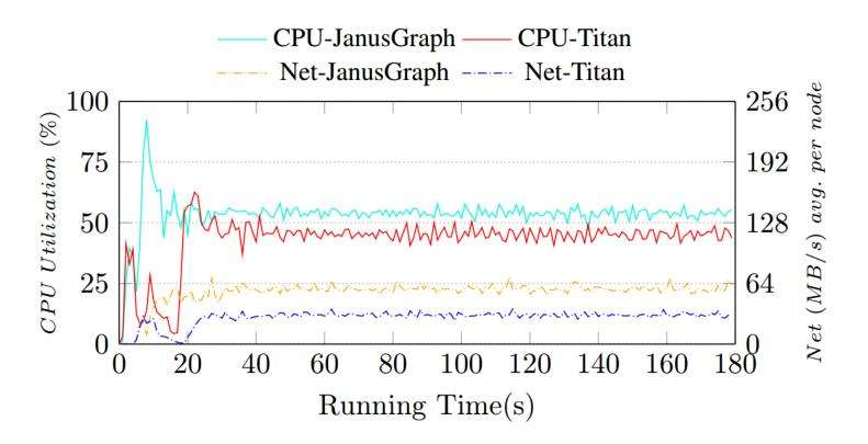
Figure 3. The CPU and network utilization for a mixed workload formed by {IS1-IS4} in LDBC benchmark.
