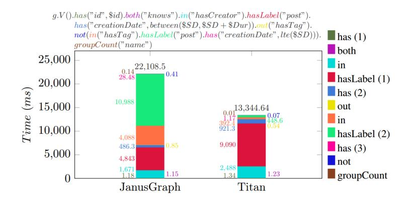
Figure 2. The query latency breakdown of IC4 in LDBC benchmark.
